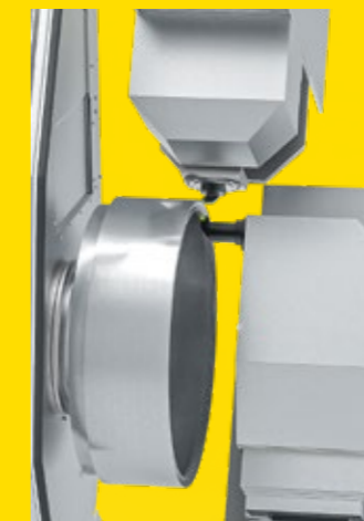
4-axis complete machining of rings
