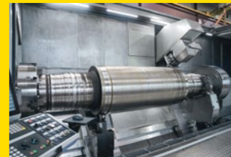
This demo part weighs around 20 tonnes and can be machined in a single clamping procedure.
