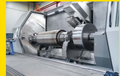
Closed working area for machining with a high coolant pressure and flow rate as well as chip removal for automatic extraction.
