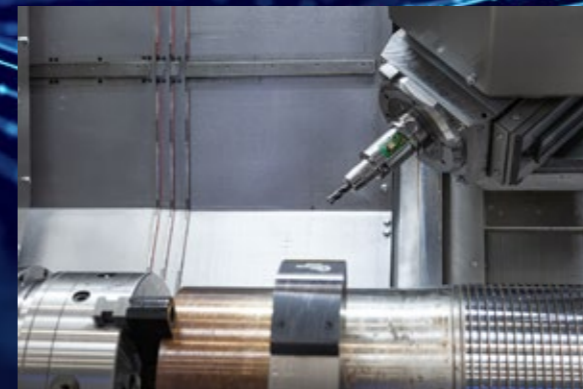
The IC0tronic Tool in operation. The machine is currently carrying out tests with a „sensored tool“, which has sensors built into the tool accommodation to allow it to communicate with the machine. The sensor technology significantly simplifies the workflow, and not only does it optimise the milling process, but it also increases the machine's productivity.
