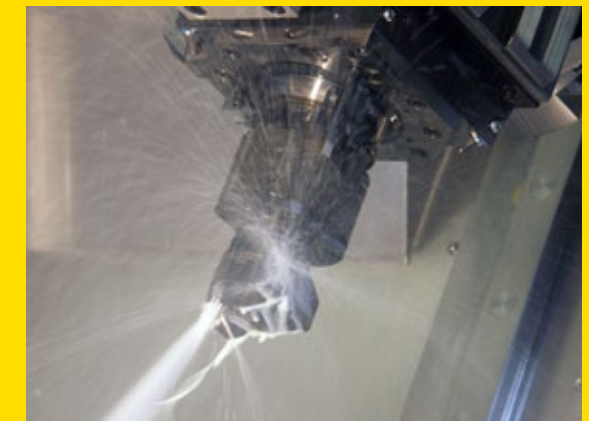
Thanks to WFL's own spindle development, the cooling lubricant can be directly fed to the cutting edge through the milling spindle at a pressure measuring up to 200 bar. This ensures rapid, continuous removal of swarf.
