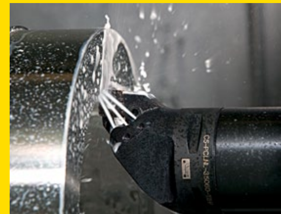
Thanks to WFL's own spindle development, the cooling lubricant can be directly fed to the cutting edge through the milling spindle at a pressure measuring up to 200 bar. This ensures rapid, continuous removal of swarf.
