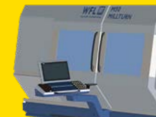
Operator panel with 220 mm height adjustment (as of M40 MILLTURN)
