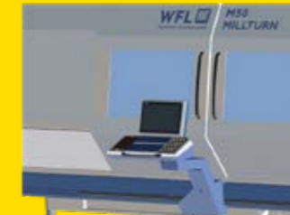
Operator panel can be swivelled around the vertical axis (105°) (as of M40 MILLTURN)
