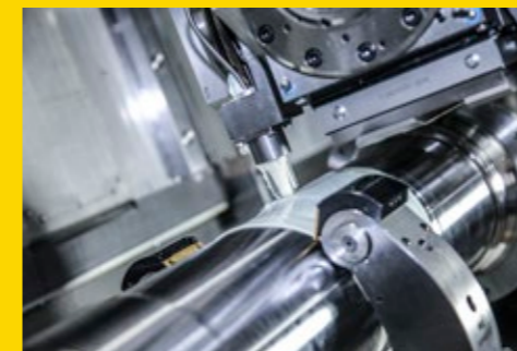
Automatic ultrasonic measurement (in-process)
