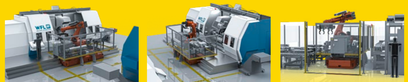
Automation with mobile robots surrounded by a safety fence to protect personnel.
