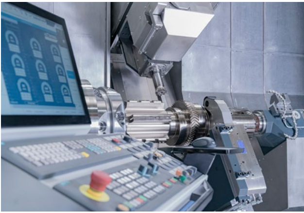
The M70 MILLTURN impresses with a well-designed working area concept for machining lengths up to 8000 mm and a swing diameter of up to 850 mm.
