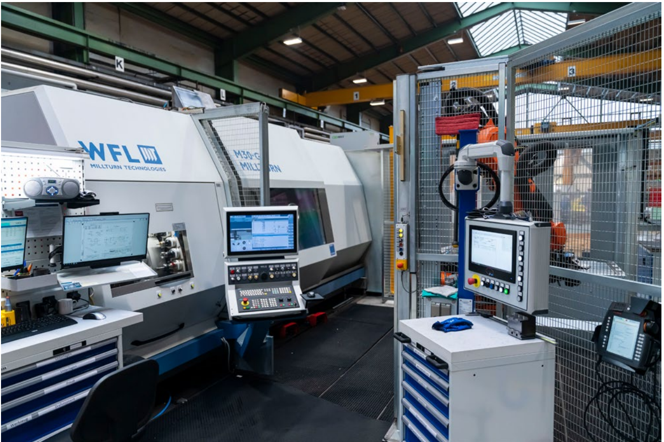
The M30-G MILLTURN with automation cell.
