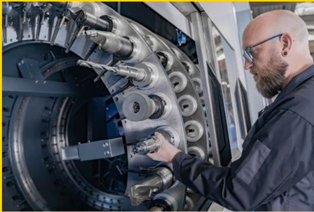
User-friendly access to the tool magazine thanks to large, easily accessible sliding window and tool set-up during machining.
