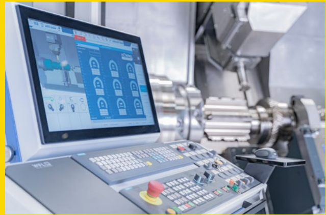
Height-adjustable, swivelling operator panel with tilttable 24-inch display.
