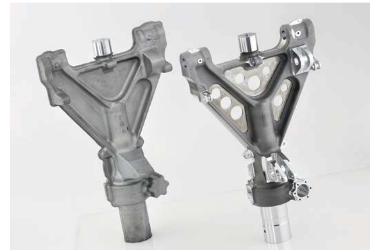
FOCAL POINT: AEROSPACE Demo version of landing gear manufactured on the M120 MILLTURN
