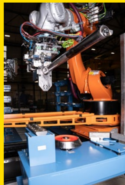
Set-up station from left to right: for prismatic tools, tailstock tips and sets of jaws
