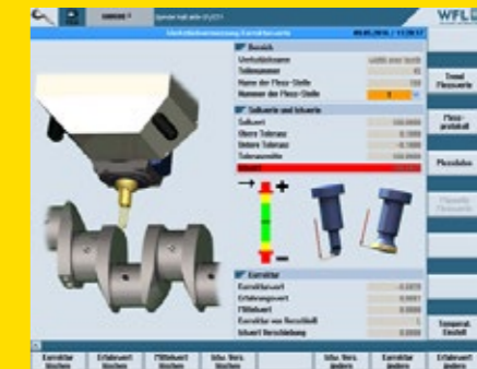
Measurements are shown (actual value, nominal value, tolerance, etc.) on the control unit display.
