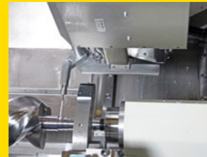
Workpiece measurement with measuring probe on the turning-boring-milling unit.
