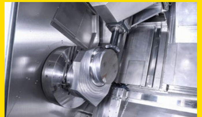
Vibration-free machining thanks to vibration damper near to the tool cutter.
