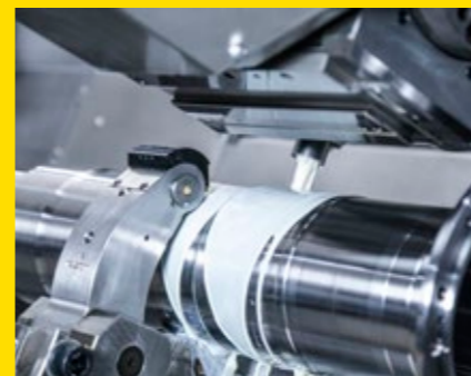
The signal for the ultrasonic wall thickness measurement is transmitted via the coolant.
