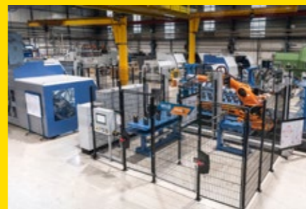
Tool and workpiece set-up station incl. HMI* and barcode scanner
