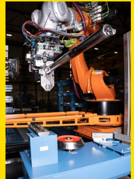
The set-up station can be used to set up tools parallel to machining time and introduce new workpieces without restricting the automation.
