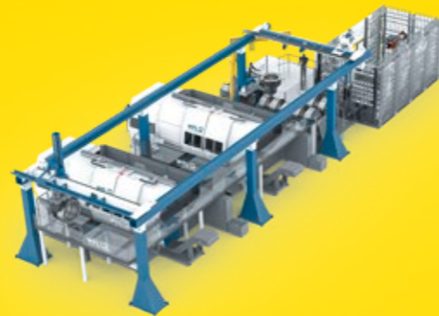
Linear and area gantry solutions consist of the same basic assemblies: gantry, set-up station for workpieces, external tool magazine (if required), buffer/lung/warehouse for multiple workpieces (optionally mounted on jigs), gripper changeover station (if required) (gripper for jigs and tools).
