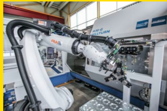
One of the most flexible automation versions of machine tools or processes is the articulated robot in a robot cell.
