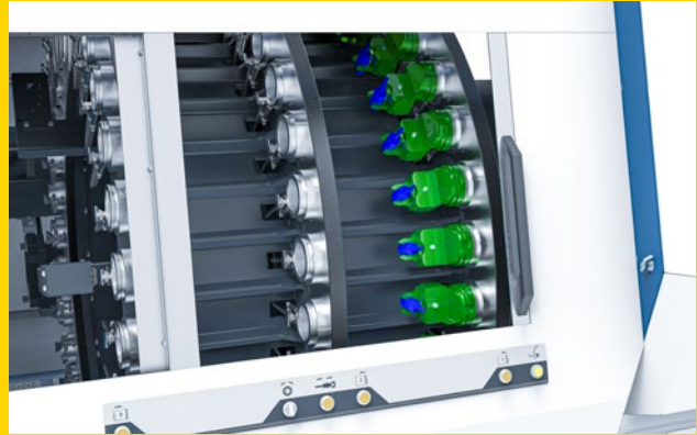
In the standard tool magazine, the various tools are stored in the adapter and can be accessed automatically.
