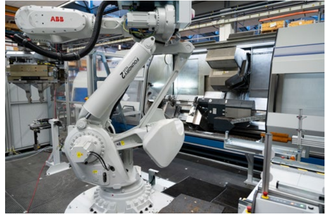
The robot with a yoke gripper is firmly anchored to the floor and is larger than usual due to the required radius between the two M65 MILLTURNs. With these dimensions, the robot can theoretically handle a load of up to 800 kg.
