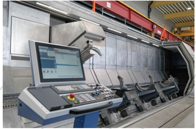
This 12-meter-long MILLTURN M100 features a special configuration designed for machining gun barrels.
