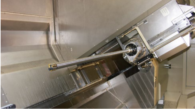
Ejector drill bits, a special form of BTA bit, are used in WFL machines at diameters of 25 mm and above.
