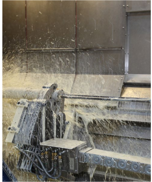
The full range of internal machining expertise from WFL. Integrated deep drilling on a Millturn complete machining centre. With a single-lip drill bit in this case.
