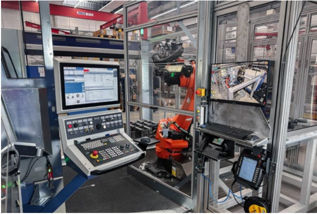
Unattended machine operation is possible with the automation cell over two full shifts.
